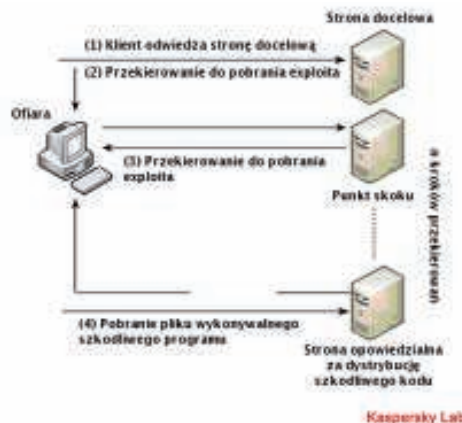
Rys. 2. Struktura ataku drive-by download
